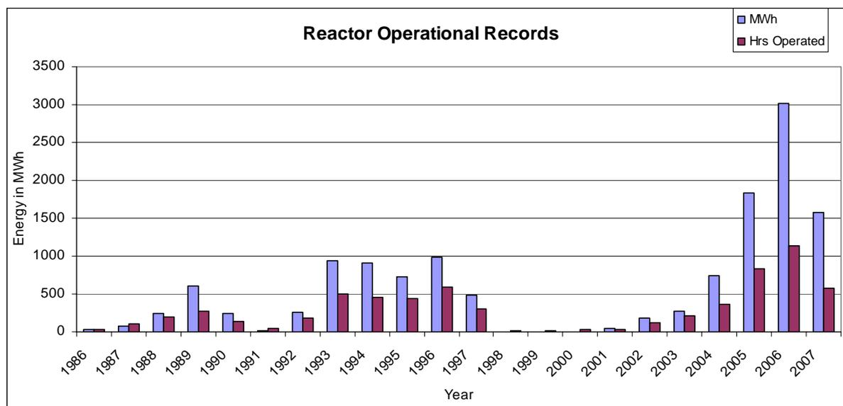
Fig.3 Operational Statistics of BAEC TRIGA Research Reactor (up to July 2007)
