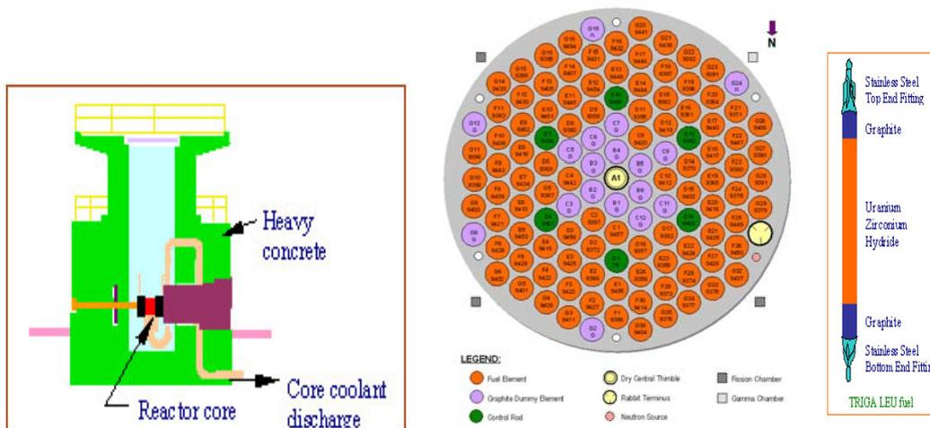
Fig.1 Sectional View of the TRIGA
