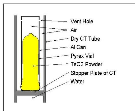
Fig. 7 Damaged Pyrex Vial inside the DCT
